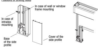
With the side profile still open, roll the blind down. If the hanging pulls down unevenly, check the side profiles for alignment and the cassette.
