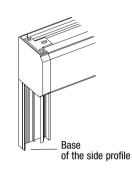
Determine no. of drilling holes in the "Base of the side profile" (depends on the surface being attached to). Place the holes in the according groove (see below). Fix the "Base of the side profile" and level up any unevenness in the surface.
