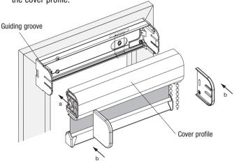
c. In case of <u>ceiling mounting</u>, remove the upper edge of the end caps as given up to the predetermined breaking point. Push the end caps onto the cover profile.
