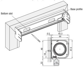
b. Fasten the fastening clips with the screws supplied.
