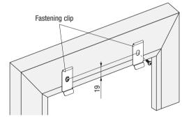
c. Clip the base profile into the fastening clips.
